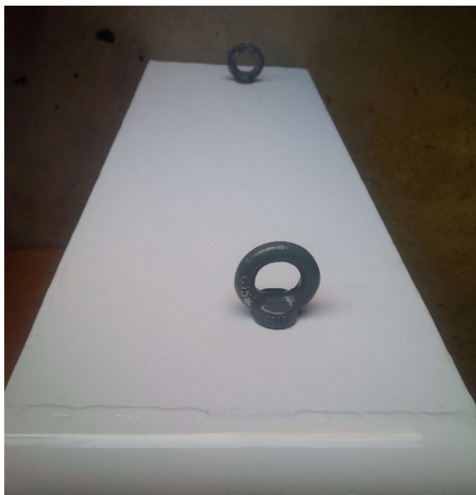
Figure 3.3 Eye bolt Installation on a 30/21 model with two eye bolts
